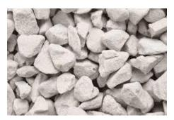
Growstones are made from recycled glass and are engineered to provide excellent drainage and aeration. They are often used in hydroponic systems.
