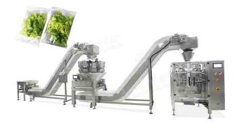
Automated bagging machines can package greens into perforated plastic bags or mesh bags, which are ideal for ensuring breathability. The system seals the bags and applies labels in one continuous process.
