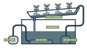
The Nutrient Film Technique involves a thin film of nutrient-rich water flowing over the roots of plants, which are typically placed in channels or troughs. The plants' roots are suspended in the air and only come into contact with the flowing nutrient solution, allowing for oxygen access.
