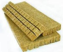
Rockwool is one of the most popular growing mediums in vertical farming. It is made by melting basaltic rock and spinning it into thin fibers, forming a lightweight material that is ideal for hydroponic systems.
