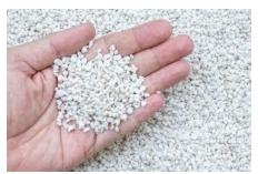
Perlite is a volcanic glass that has been heated and expanded to create lightweight, porous particles. It is frequently used in combination with other grow mediums, like coco coir or vermiculite, to enhance drainage and aeration.
